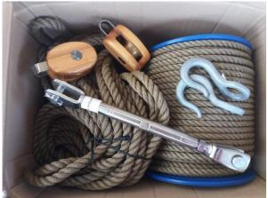
Its contents: 150 meters of new SPUNFLEX rigging (ropes) of two different strengths, 4 large 2-sheave blocks for the rope hoists, small single-sheave blocks for new halyards, rigging hooks, shroud tensioners, hardwood corals, 10 liters of BENAR oil, UVR-resistant wood coating, rigging twine, and much more.
